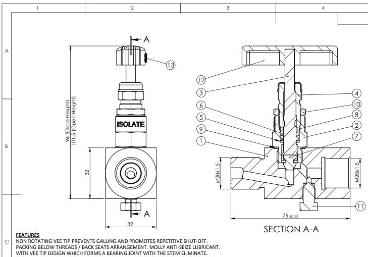
PART NO. PART NAME Material QTY. ASTM A479 SS316 Body 2 Gland Body ASTM A479 SS316 3 ASTM A479 SS316 Stem 4 Retainer ASTM A479 SS316 5 **Bottom Washer** ASTM A479 SS316 6 Packing PTFE 2 7 Vee Tip ASTM A564 SS174 8 Top Washer ASTM A479 SS316 9 Thrust Ring ASTM A240 SS316 ASTM A479 SS316 10 Check Nut 11 Drain Plug ASTM A479 SS316 12 ASTM A351 CF8M Handle
